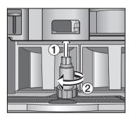
■ Using the special tool (supplied) as shown above, turn the capsule hopper anti-clockwise to remove it.
